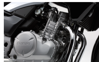
Liquid-cooled, in-line 2-cylinder
